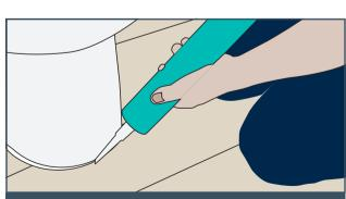
11. For splash areas such as bathrooms, waterproof skirting/scotia/trims can be used. Cut the flooring around your WC base leaving a 8-10mm expansion joint. 100% silicone sealant can be used around the expansion gap of a WC or small wet areas (sink pedestall), but cannot be used in large areas as this will restrict the expansion and contraction of the tiles and cause the joints to fail.
