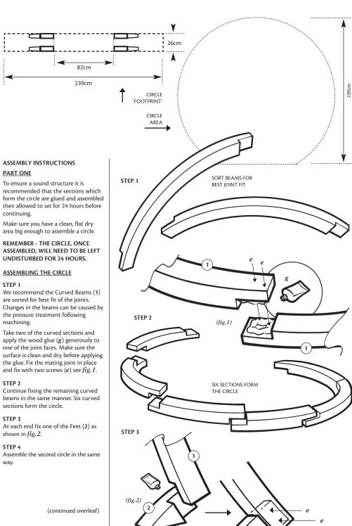
recommended that the sections which form the circle are glued and assembled then allowed to set for 24 hours before continuing.
