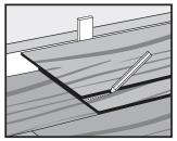
Remove spacers. Cover expansion spaces with quarter round or other trim, being sure not to trap or pin down the floor. Nails should go into wall, not
