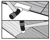
After installing the last piece of the second row, slide the entire assembly against the spacers on the starting wall, maintaining the
