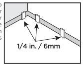
2 Loose lay the first row of planks in order to obtain a better visual of the installation and to avoid having a plank less than 20.3cm (8") on the opposite end of the room. If you end up with a plank less than 20.3cm (8"), cut the first plank accordingly to properly balance the room.
