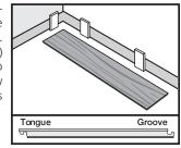
Interlock the next plank at the end joint of the first plank by inserting the tongue into the groove of the adjoining planks.
